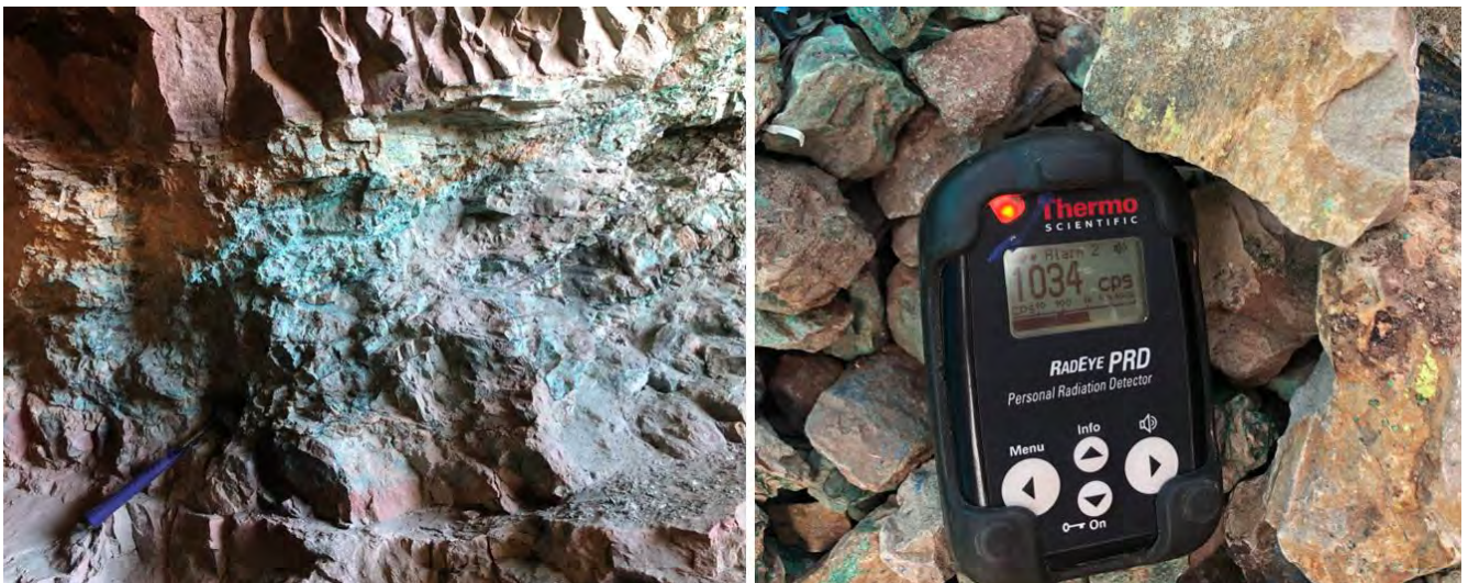
Figure 5-8. Left: Ore lens exposed within a drift within the excluded zone on permit 3942217, site of channel samples AR-CH01 and AR-CH02. Right: Secondary Cu and uranium (yellow minerals) from a stockpile from Bou Anas (not on the Project).
